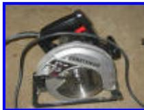
The circular saw. If you don't have access to a table saw, this will serve you almost as well. I have a plywood cutting blade in it, which does a very nice job with my cuts. This blade will also cut laminate.
