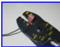
J) Squeeze the end a bit to tighten it
