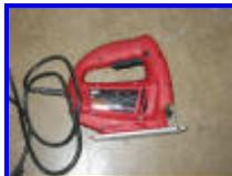
The jig saw. It is handy for cutting the first side. Run it against a straight edge and the resultant cut is nearly impossible to discern (by sight) from a circular saw cut. The downside is it takes a lot longer to cut with than the other saws.
