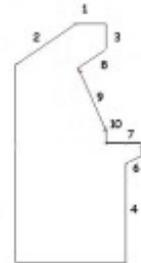
The first cut (#1) was made with the circular saw. I cut the excess material from the top of the board. I lined the cut up with the very top of the cabinet (72" from the base). See picture C.
