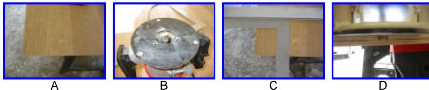
I started about an inch in from the left edge. I started the router up and slowly (keeping the router against the straightedge) brought it down into the wood. It'll take a second for the bit to chew through the wood. Once the router base is flat against the plywood side, slowly cut to the right. You might need to stop a couple times to clear all the dust from the slot- you are cutting a fair amount of wood here. Stop when the router bit reaches the
