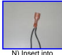
N) Insert into disconnect and crimp with cutter (as in J)
