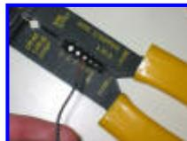
F) About 3/4" of wire being stripped of the insulation
