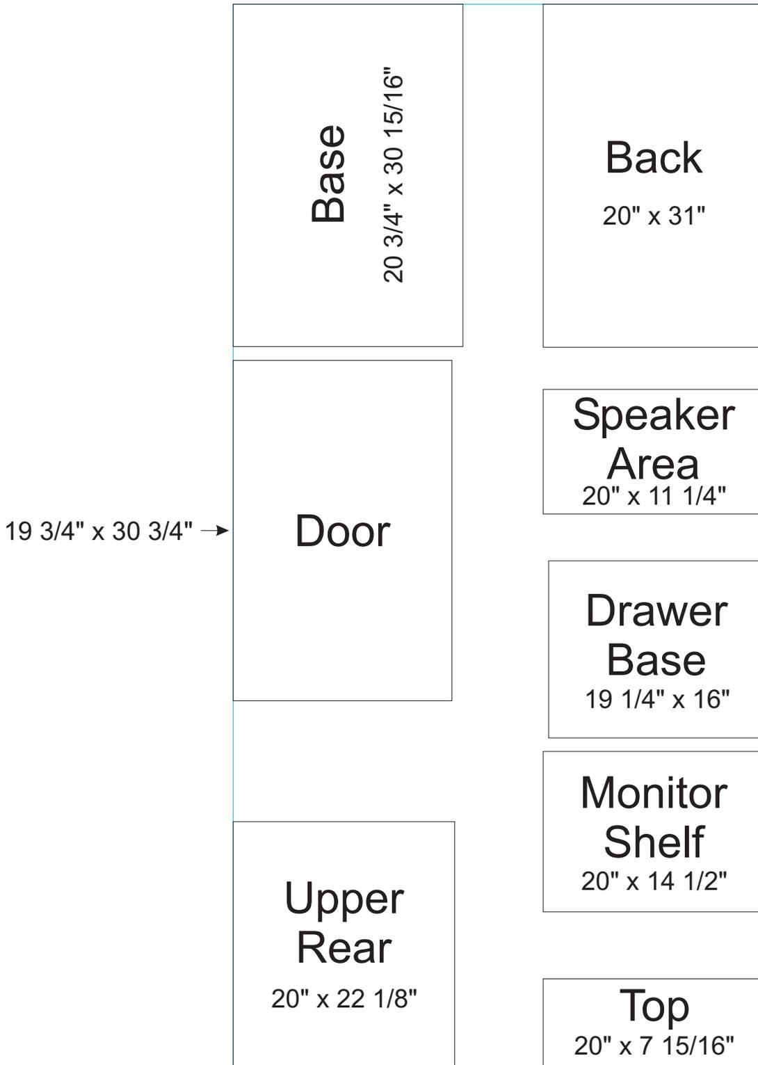
Use this layout for sheet 3 if you are making a partial back cabinet and do not use the cutout for the Upper Rear on sheet 1
