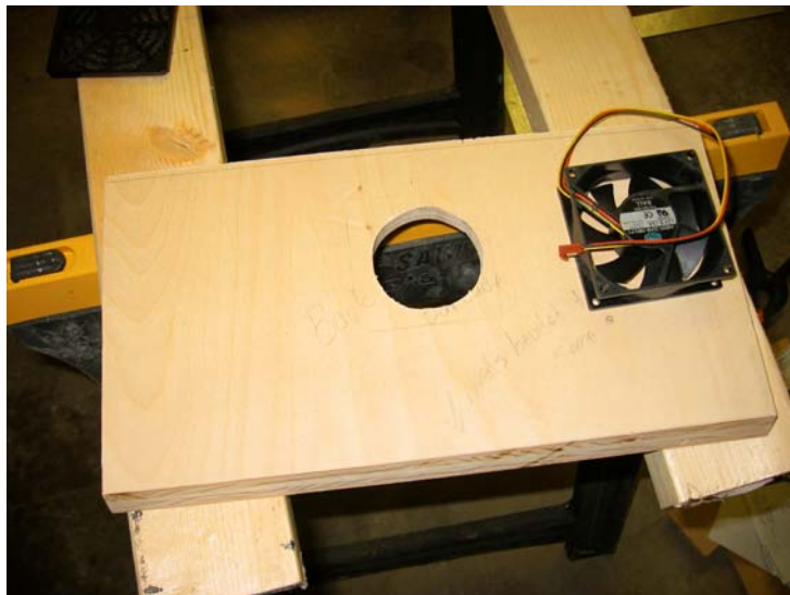
Figure 12- The hole has been cut for the fan
