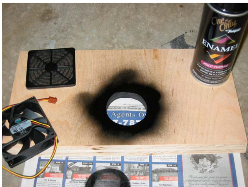
Figure 13- The inside of back panel, after spray painting
