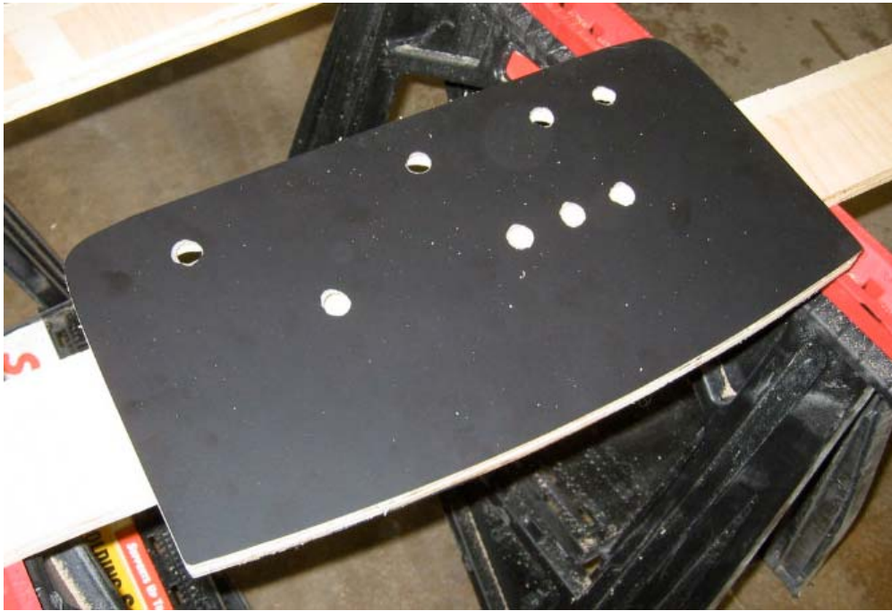
Figure 30 - Button holes are pre-drilled
