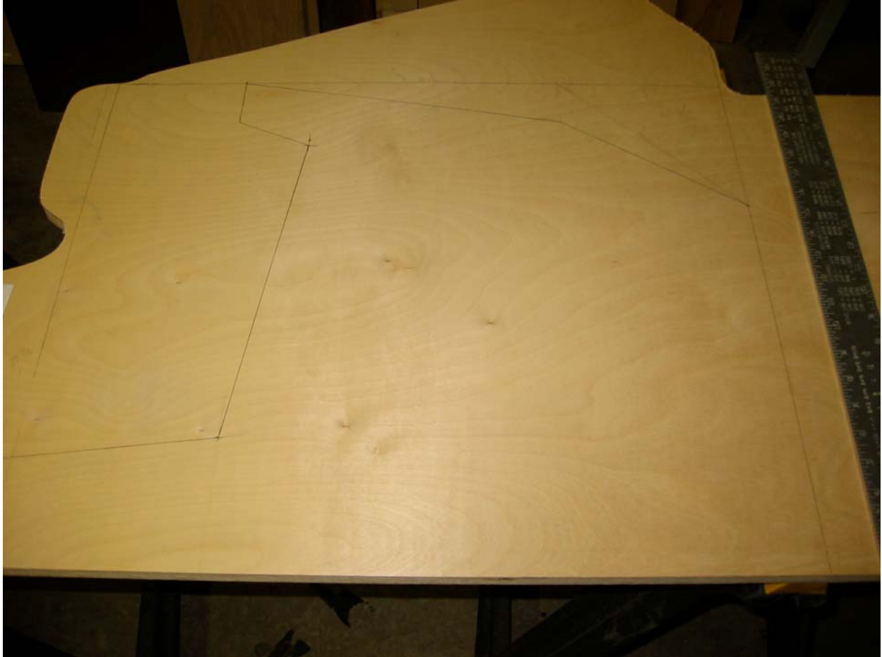
Figure 2: Side S1, with outline drawn on wood
