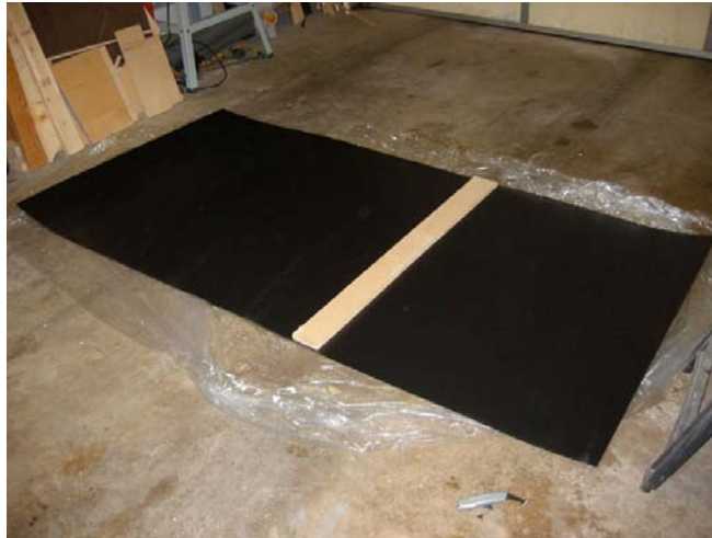
Figure 27 – Laminate sheet prior to scoring
