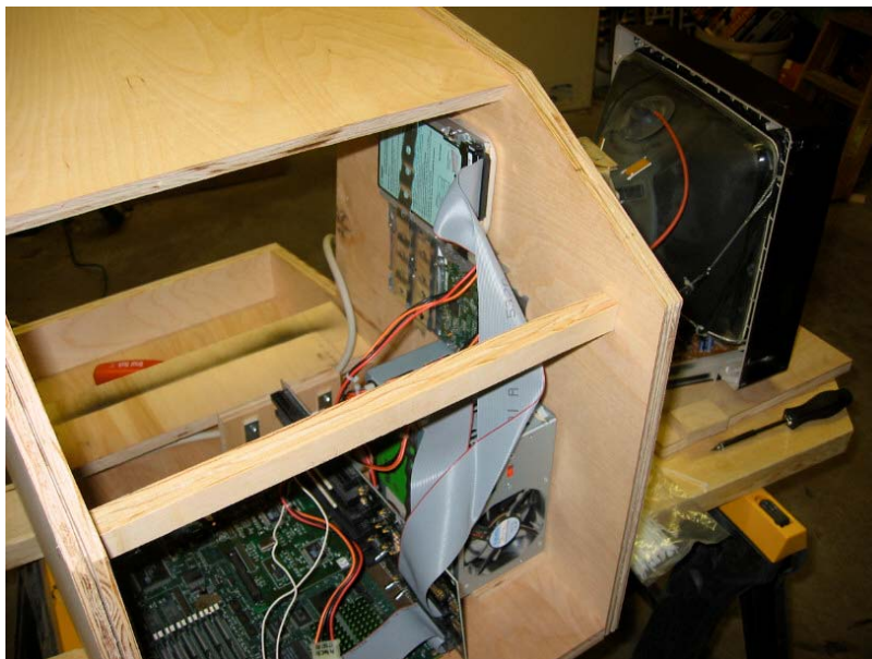
Figure 20 – Hard drive and diskette drive in place
